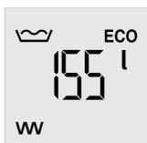
The currently available mixed water volume at 40 °C and at 15 °C cold water temperature is shown.
