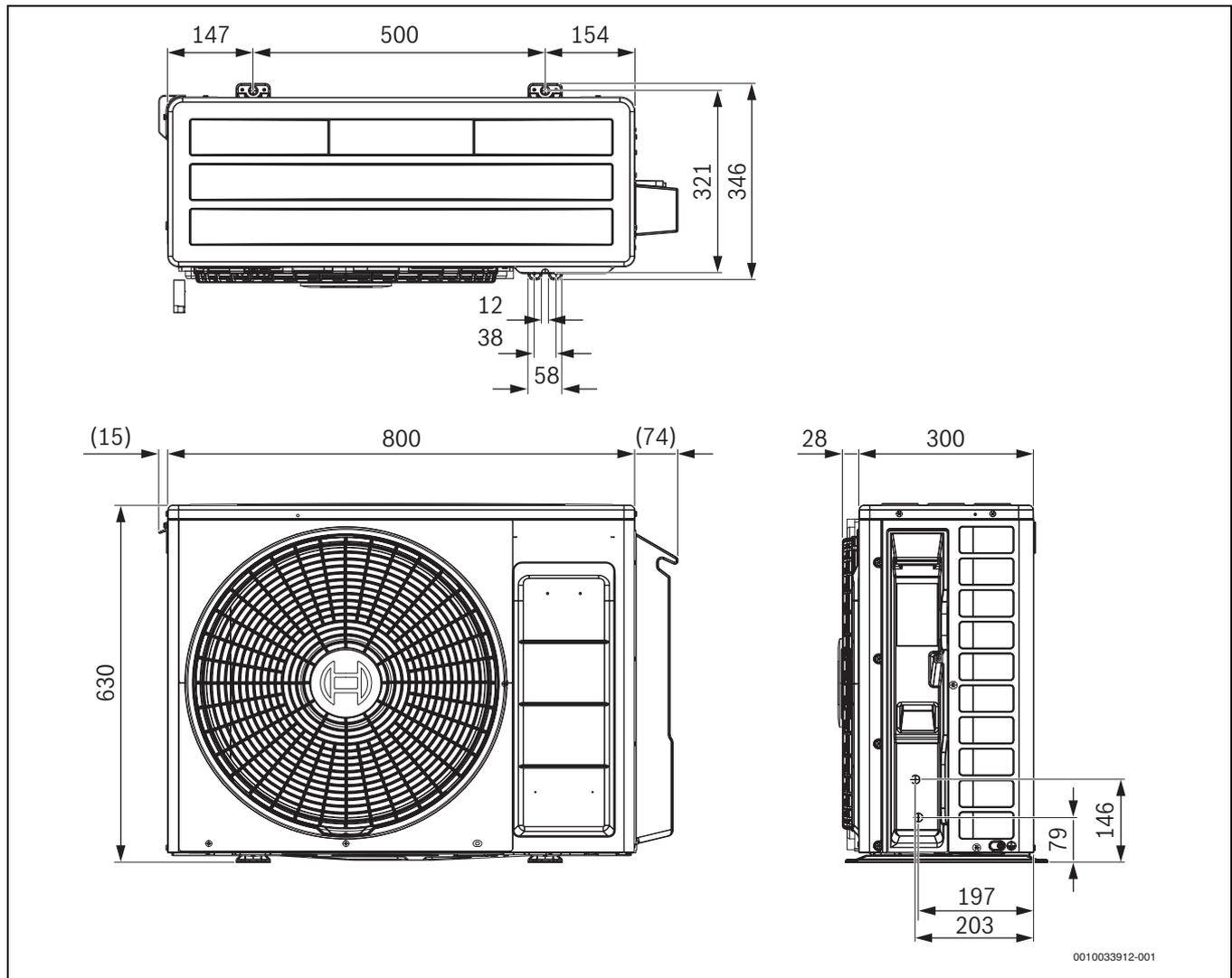
Fig. 2 Outdoor unit dimensions - (in mm)
