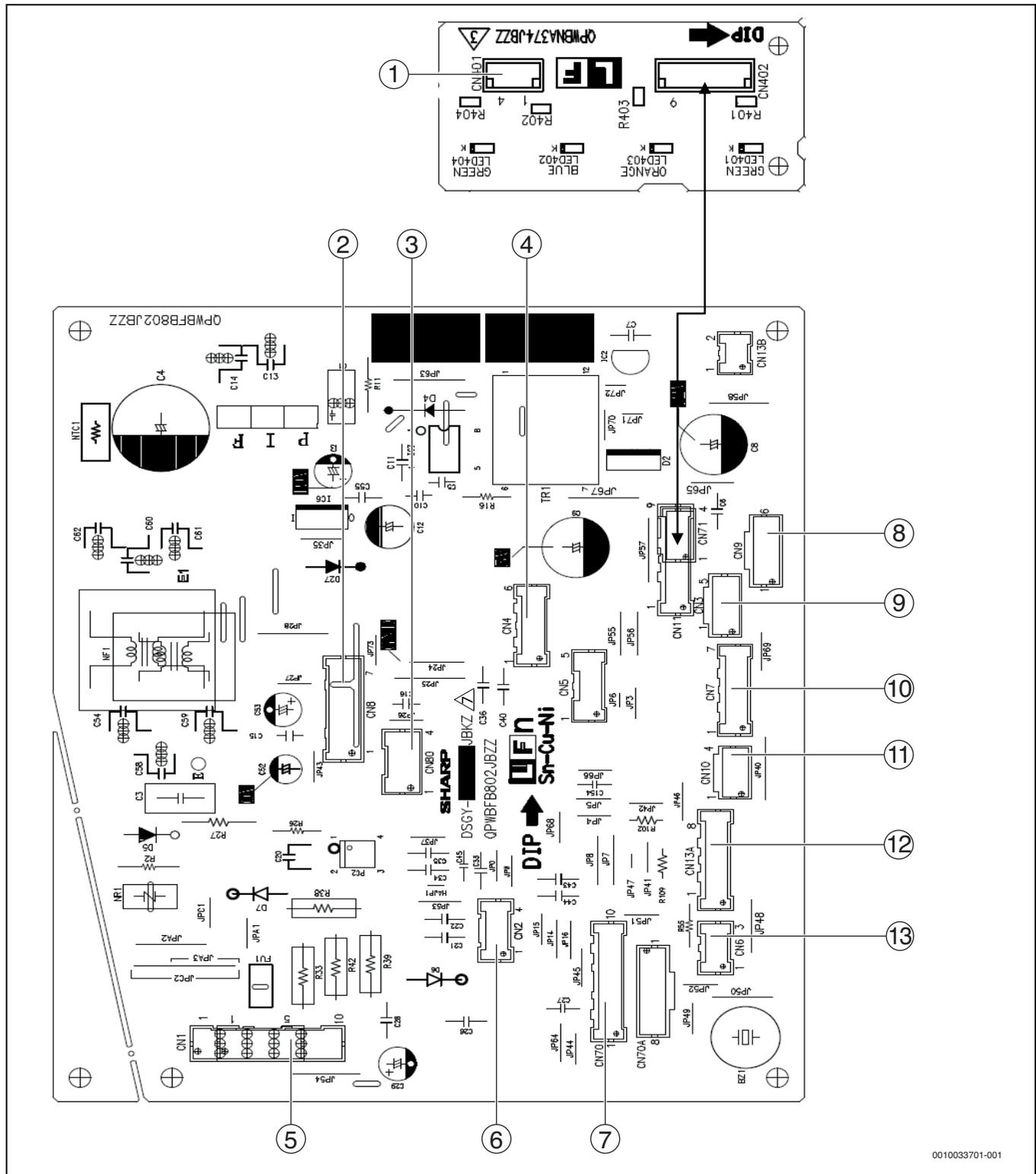
Fig. 6 Indoor unit wiring
