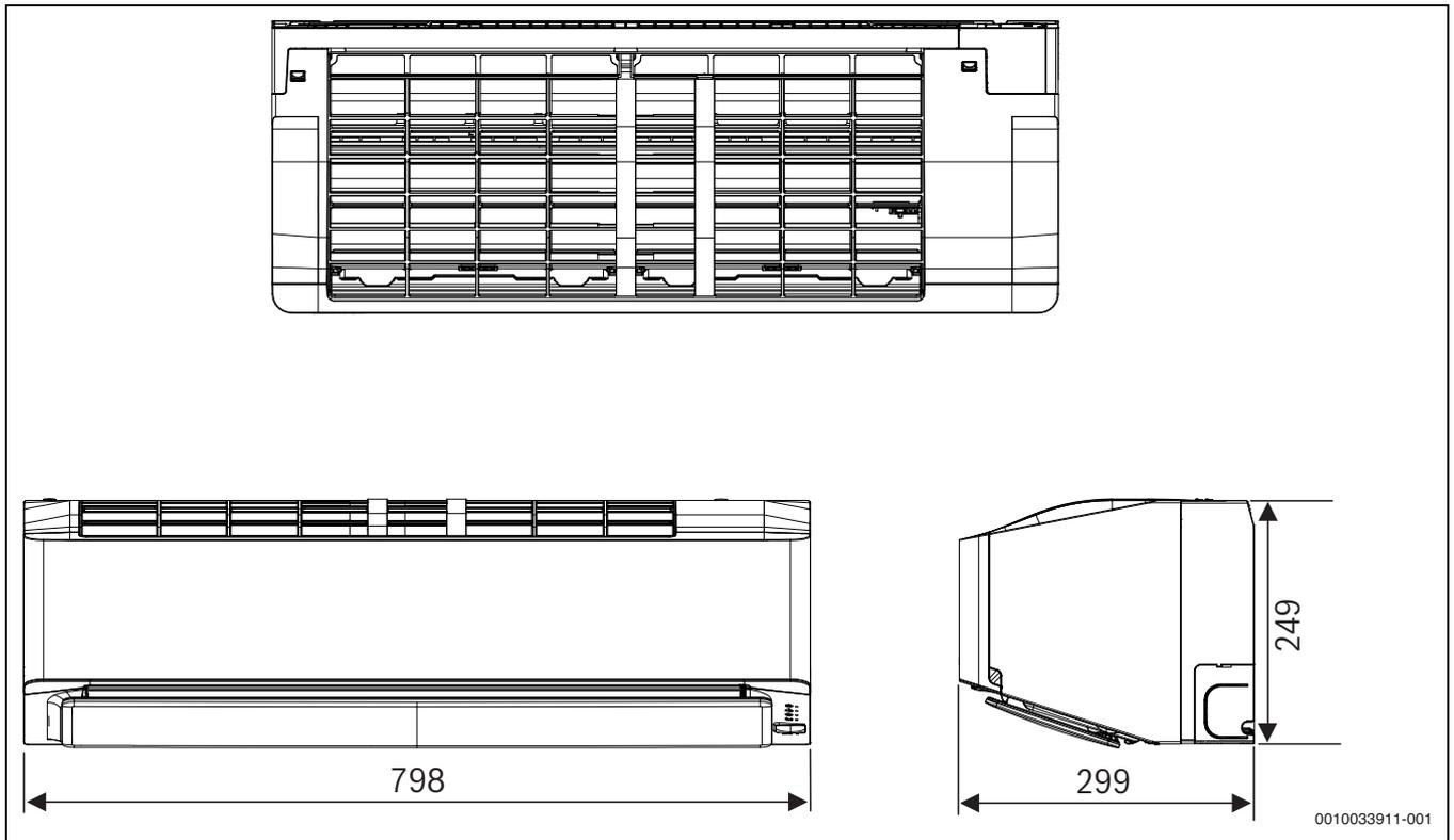
Fig. 1 Indoor unit dimensions (in mm)
