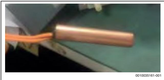
Fig. 132 Pipe thermistor
