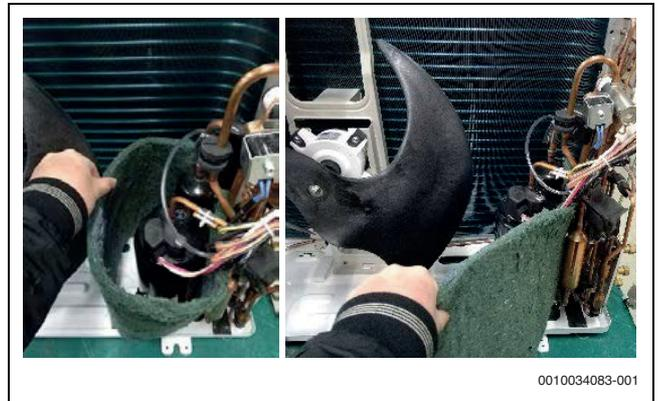
Fig. 109 Removing compressor cover 2
