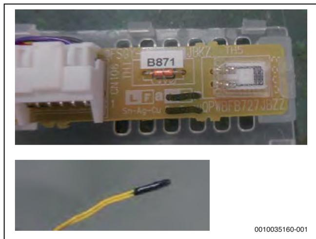
Fig. 131 Room temperature thermistor
