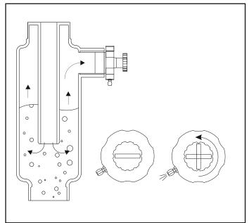
**Venting**To vent the system, turn the hand vent knob until fluid flows out through the vent.
