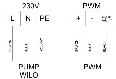
\*if the controller to which the PWM signal is connected is not able to read the return signal, leave the black cable disconnected.
