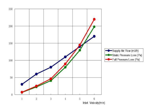
Remarks: 1.Above Table, Pressure Loss Included Resistance caused by 7 Leafs and Wire Net
