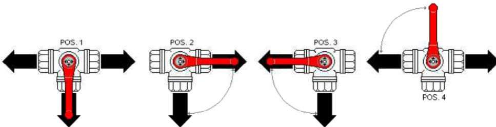
TO OBTAIN THE POSITION 3 AND 4, REMOVE THE LEVER FROM THE PUSHROD!
