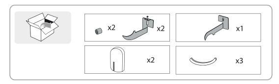
**WARNING:** the screws and dowels are not provided with the packaging, so please use screws and dowels that are suitable for the type of wall material the radiator is to be fixed to. The dowel must have a 10 mm diameter, the screw must have a 60 mm length, a 7,5 mm diameter and an hexagonal head.
