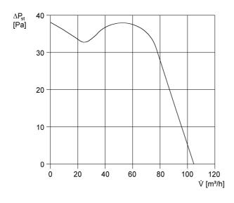
U = 230 Vf = 50 Hz n = 2500 min<sup>-1</sup>
